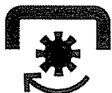
ATTACHMENT CLUTCH ENGAGED
